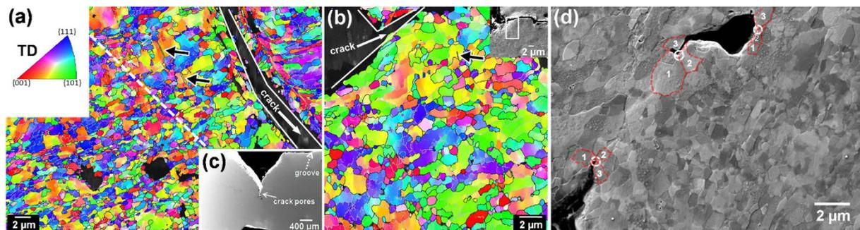
**Figure 6. Microstructure characterization of crack section in impacted ECAP-16 Cu sample.** (a,b) OIM images near cracks of the ECAP-16 Cu sample. (c) SEM image of impact fractured specimen. Black lines indicate boundary mis-orientation  $>15^\circ$ , and grey lines indicate mis-orientation between  $2^\circ$  and  $15^\circ$ . (d) SEM image of secondary impact cracks and voids near the main crack of the ECAP-16 Cu sample. Numbered red circles mark the grains around the triple junction.
