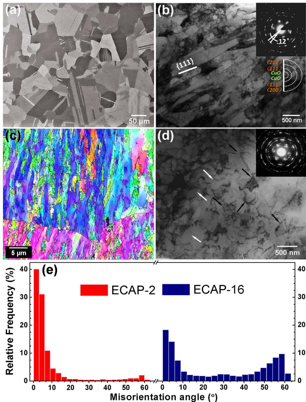
**Figure 1. Microstructure characterization of Cu samples.** (a) Microstructure of initial CG Cu after annealing; (b) TEM micrograph of the UFG Cu after ECAP processing for 2 passes. The inset is SAED with a selected area of 5 μm in diameter, (c) EBSD map of grain orientation of ECAP-2 Cu. (d) TEM micrograph of UFG Cu after ECAP processing for 16 passes. The inset is SAED with a selected area of 5 μm in diameter. (e) Distribution of boundary mis-orientation angles measured using EBSD.
