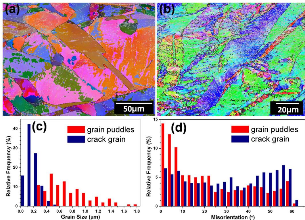
**Figure 5.** EBSD characterization of ECAP-2 Cu sample with initial grain puddles and impacted crack grains. (a,b) OIM images of ECAP-2 sample with different magnifications. Frequency distributions of (c) grain size and (d) GB mis-orientation of as-ECAPed grain puddles and as-impacted near-crack grains.
