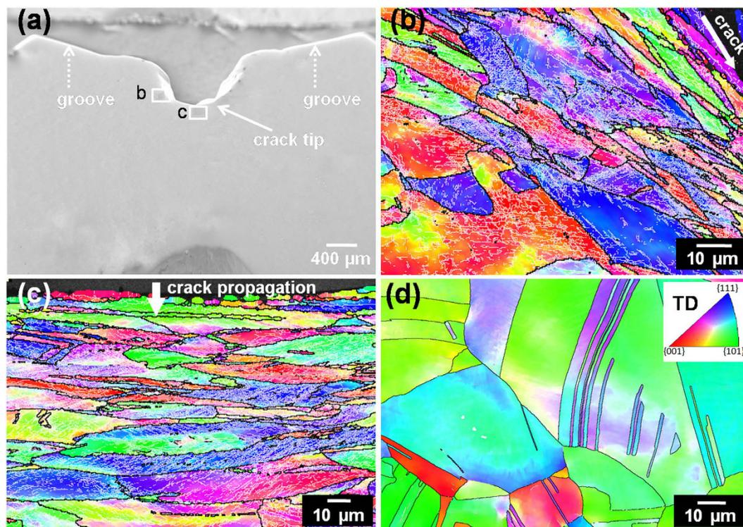
**Figure 3. Microstructure characterization of crack section in impacted CG Cu sample.** (a) SEM image near the crack of a CG Cu sample. (b,c) OIM images of grains near the crack edge and tip, respectively. (d) OIM image of grains far away from the crack. Black lines indicate boundary mis-orientation  $>15^\circ$ , and grey lines indicate mis-orientation between  $2^\circ$  and  $15^\circ$ .
