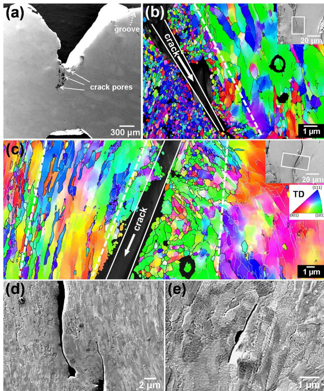
**Figure 4. Microstructure characterization of crack section in impacted ECAP-2 Cu sample.** (a) SEM image of impacted ECAP-2 Cu sample, (b) OIM image of grains near crack tip, (c) OIM image of grains along the crack edge. Black lines indicate boundary mis-orientation  $>15^\circ$ , and grey lines indicate mis-orientation between  $2^\circ$  and  $15^\circ$ . (d,e) SEM images of small secondary cracks near the main crack of the impacted ECAP-2 Cu sample.
