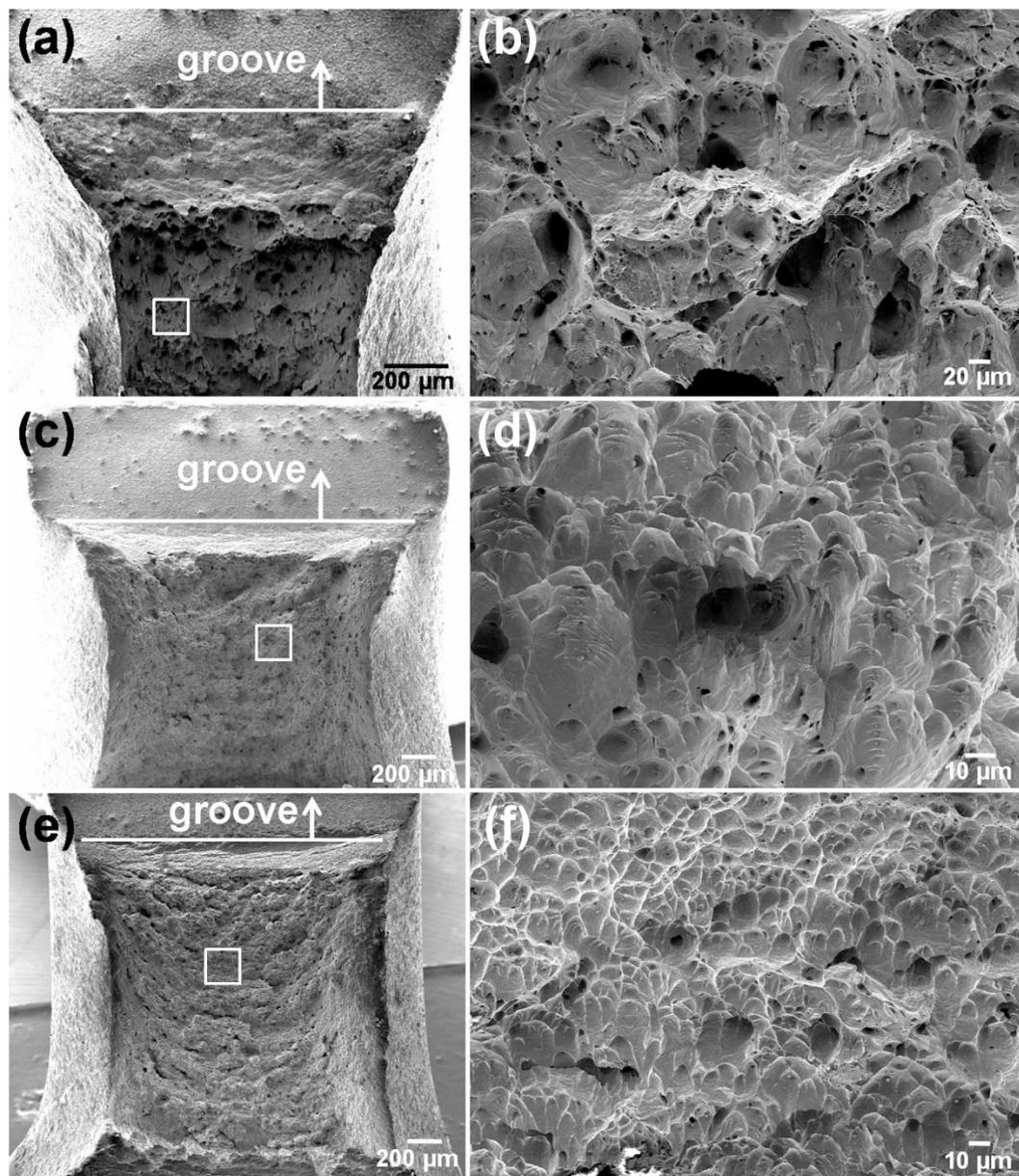
**Figure 7.** SEM observations of the impact fracture surfaces. CG Cu (a,b), ECAP-2 Cu (c,d), and ECAP-16 Cu (e,f). (b,d,f) are the magnified images of marked area in (a,c,e), respectively.
