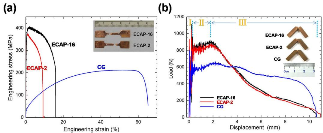
**Figure 2. Mechanical properties curves of Cu sample.** (a) Tensile engineering stress-strain curves of the UFG (ECAP-2 and ECAP-16) and CG Cu at a strain rate of  $1 \times 10^{-3}$ . (b) Load-displacement curves of the UFG (ECAP-2 and ECAP-16) and CG Cu under Charpy notched impact tests at room temperature. The strain rate is  $1.3 \times 10^3 \text{ s}^{-1}$ . Insets show the impacted specimens.
