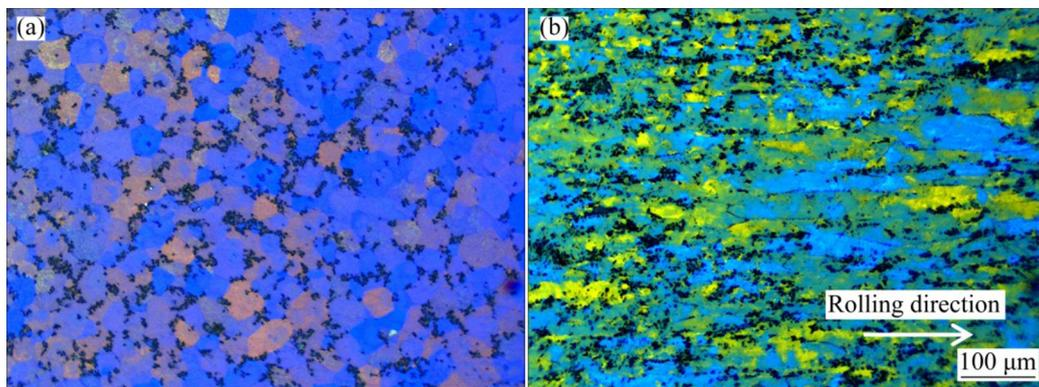
**Fig. 4** Polarized light optical micrograph of Al–TiB<sub>2</sub>/TiC in situ composites: (a) As-cast; (b) After rolling with 90% reduction
