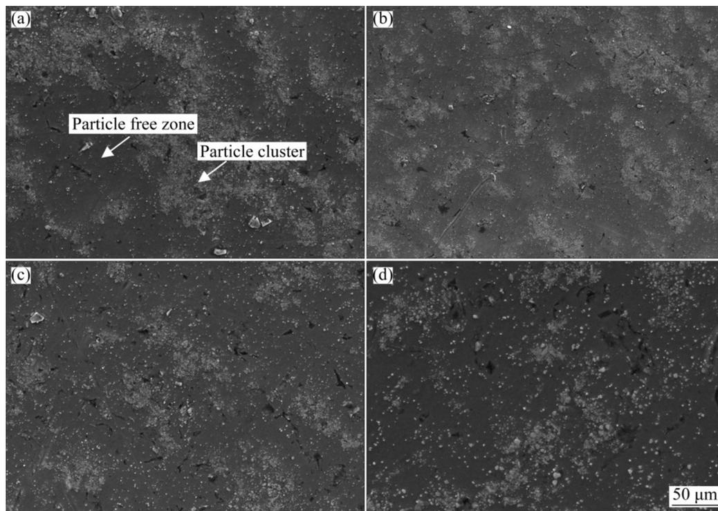
**Fig. 2** Microstructures of Al–TiB<sub>2</sub>/TiC in situ composites with different rolling reductions (in RD–TD plane): (a) 20%; (b) 40%; (c) 80%; (d) 90%
