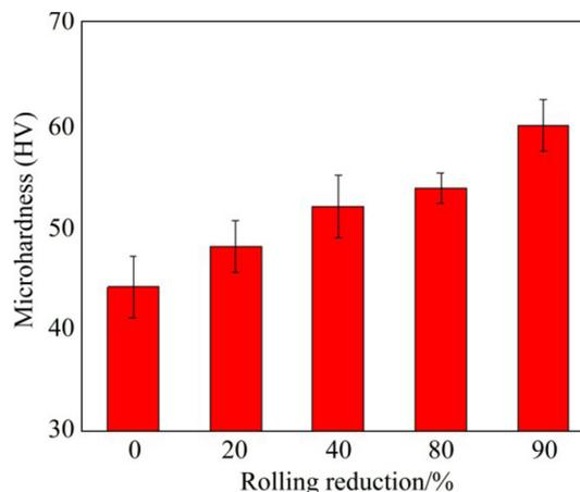
**Fig. 6** Variation of microhardness of Al-TiB<sub>2</sub>/TiC composites vs rolling reduction
