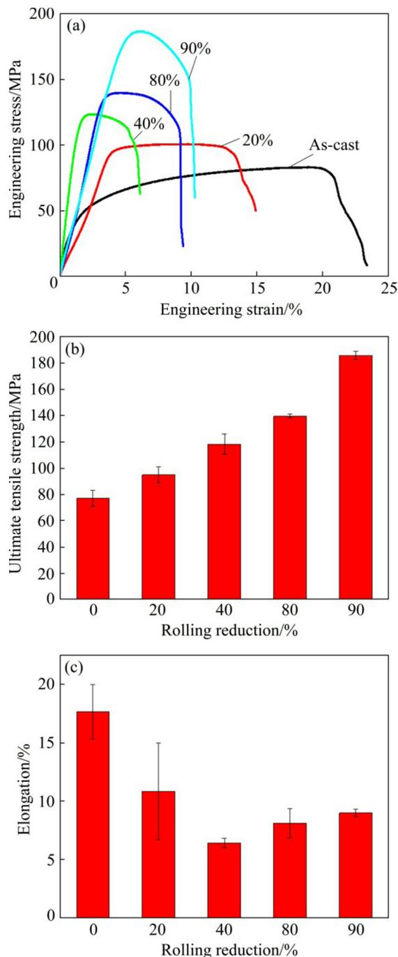
**Fig. 5** Tensile properties of Al-TiB<sub>2</sub>/TiC composites with different rolling reductions: (a) Engineering stress-strain curves; (b) Variation of UTS vs reduction; (c) Variation of elongation vs reduction
