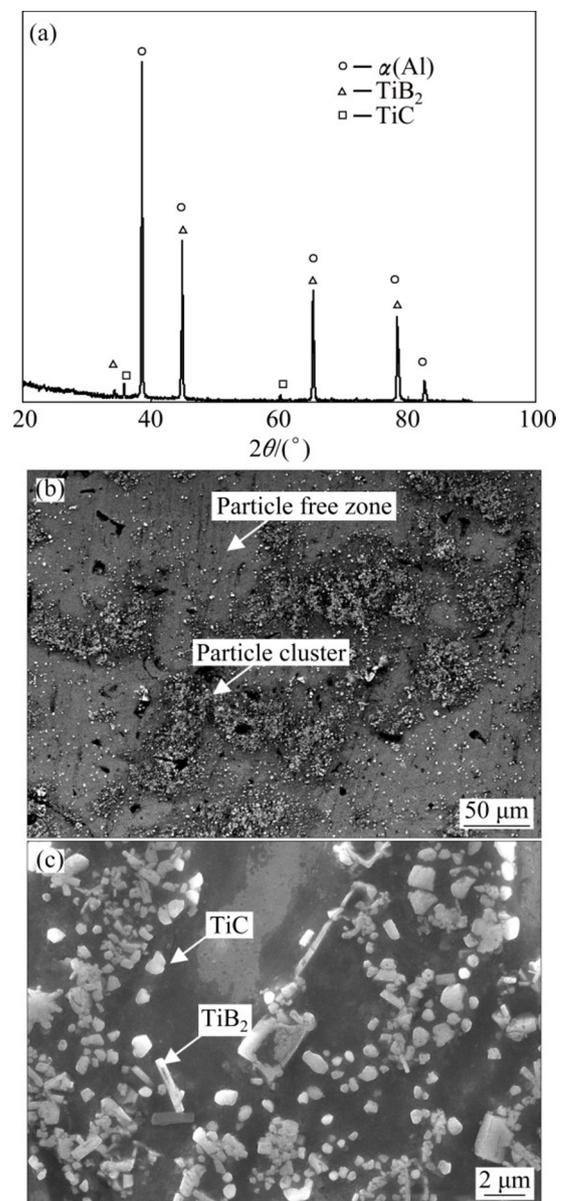
**Fig. 1** XRD pattern (a) and FESEM micrographs at low (b) and high (c) magnification of Al–TiB<sub>2</sub>/TiC in situ composites
