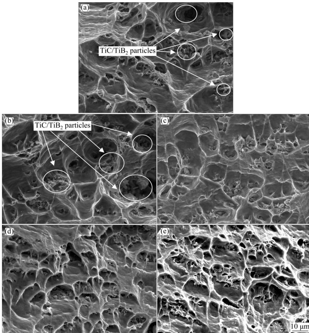
**Fig. 7** Fractographs of Al–TiB<sub>2</sub>/TiC composites in as-cast state (a), and after rolling with 20% (b), 40% (c), 80% (d) and 90% (e) reduction
