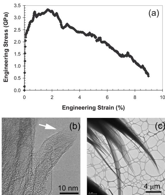
**Figure 4.** a) Stress–strain curve of a CNT fiber under tension shows non-brittle behavior. b) TEM image shows broken CNT ends (marked by an arrow) after tensile testing. c) TEM image of the fracture morphology of a CNT fiber indicates sliding between CNT strands. The background in (c) is supporting carbon foil.
