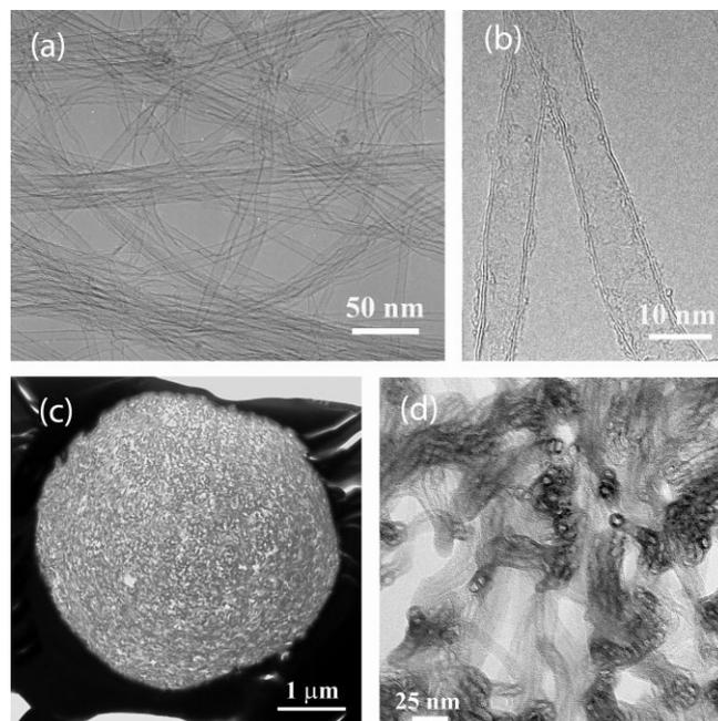
**Figure 3.** a) TEM image showing CNTs with relatively large diameters and thin walls, b) high-resolution TEM image revealing the CNTs as double-walled, c) TEM image showing the cross section of a CNT fiber encased in platinum (the black surrounding), and d) enlarged area from (c) showing the low packing density of the CNT fiber. The circles are where CNT strands exit the specimen top or bottom surfaces.
