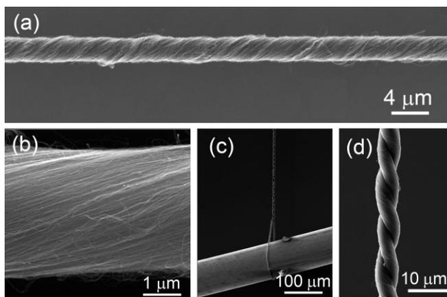
**Figure 2.** SEM images of CNT fibers. a) CNT fiber at low magnification. b) CNT fiber at high magnification. c) CNT fiber forming a loop around a Ni wire and then twisted. d) Twisted two-ply section of the fiber in (c).
