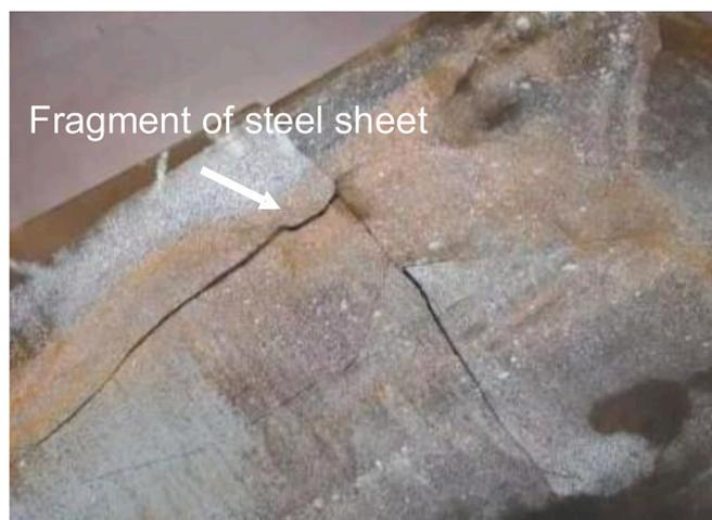
Fig. 1. Quench-cracked boron steel sheet with a thickness of 6 mm.
