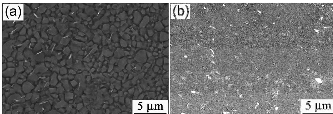
**Figure 3.** Bright-field SEM images of the microstructure of Mg-Zn-Ca after HPT+annealing at 200 °C: (a) average grain size; (b) size of second-type particles.
