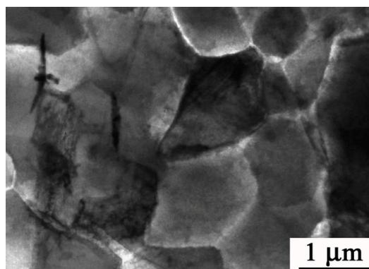
**Figure 4.** TEM microstructure of Mg-Zn-Ca after HPT+ annealing at 200 °C.
