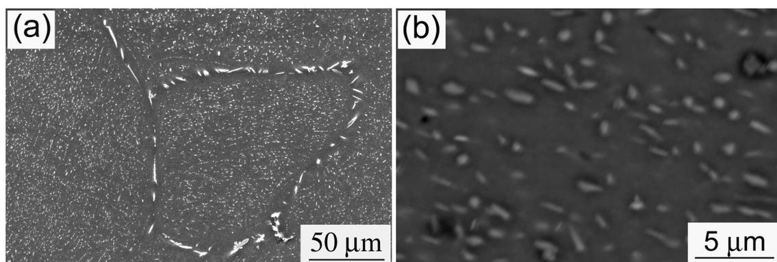
**Figure 1.** Initial structure of Mg-Zn-Ca: (a) first-type particles – in grain boundaries; (b) second-type particles – in grain bodies.
