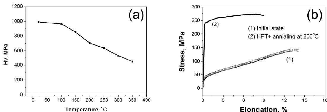
**Figure 5.** (a) – change of microhardness of Mg-Zn-Ca after HPT depending on the annealing temperature; (b) - tensile tests of Mg-Zn-Ca at room temperature and a strain rate  $10^{-3} \text{ s}^{-1}$ : (1) initial coarse-crystalline state, (2) after HPT and additional annealing.
