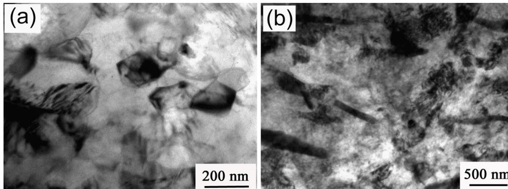
**Figure 2.** Bright-field TEM images of the microstructure of Mg-Zn-Ca after HPT: (a) average grain size; (b) size of second-type particles.
